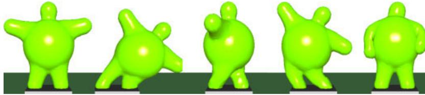
Figure 1. Object main modes. From left to right: rest position, 2nd, 3rd, 5th, and 7th mode.
