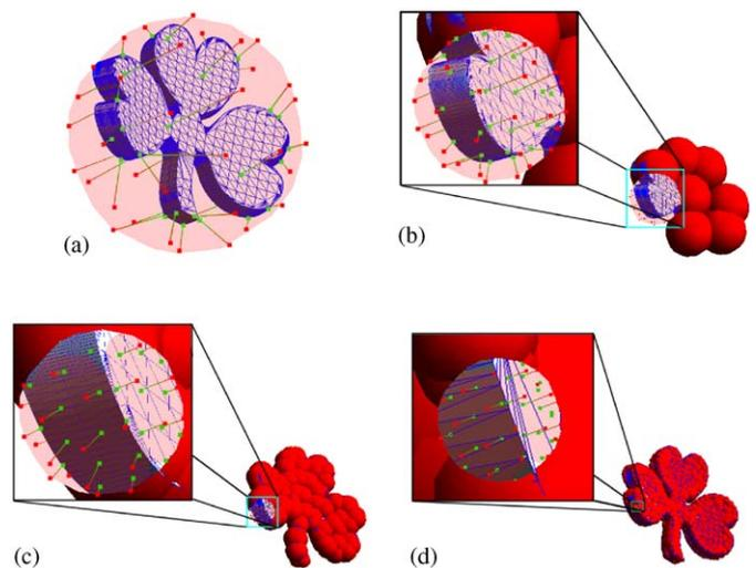
Fig. 2. Closest feature map of four sphere-tree levels for a shamrock model: (a) top level; (b) level 2; (c) level 3; (d) level 4.
