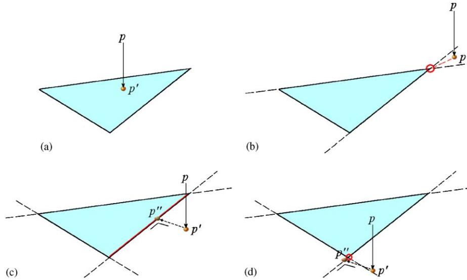
Fig. 4. Different cases that can be encountered during closest point searching: (a) point inside triangle; (b) outside triangle in front of two edges; (c) in front of one edge and inside triangle; (d) in front of one edge and outside triangle.
