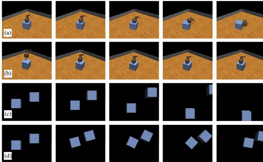
Fig. 6. Two example scenes illustrating CFM approach improving contact response for worse case scenarios: (a) non-CFM approach—bunny landing on top of another box; (b) CFM approach—bunny landing on top of another box; (c) non-CFM approach—resolving collisions at highest spherical level; (d) CFM approach—resolving collisions at highest spherical level.
