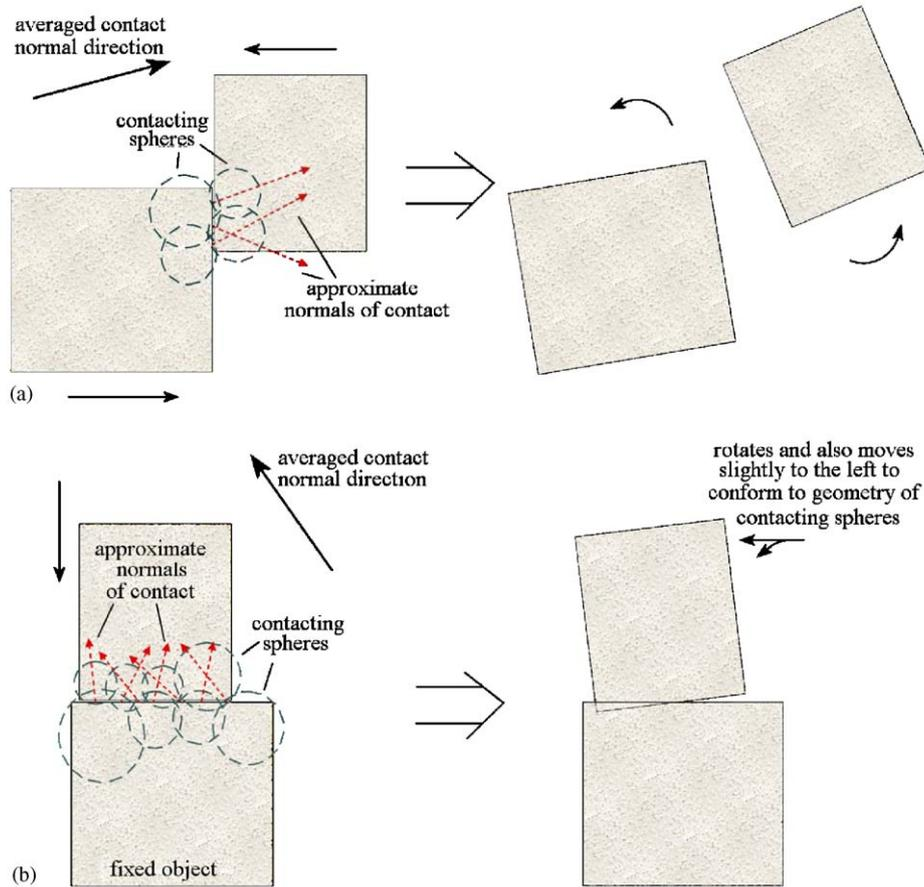
Fig. 1. Cases where over-approximation of contact data is appropriate and inappropriate: (a) normal approximation does not affect overall plausibility of object response; (b) inaccurate contact normals cause unwanted rotation and shifting during response.
