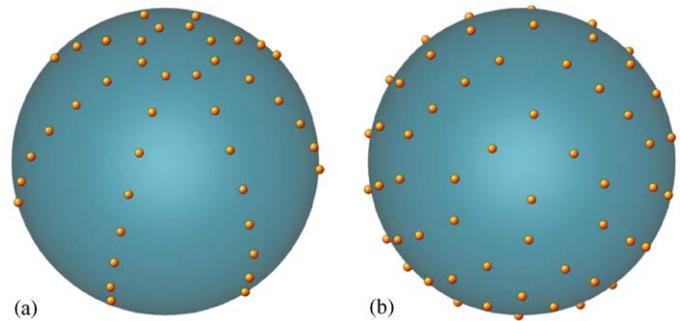
Fig. 3. Difference in point distribution for non-adaptive and adaptively created polar sample points: (a) normal polar sampling; (b) adaptive polar sampling.
