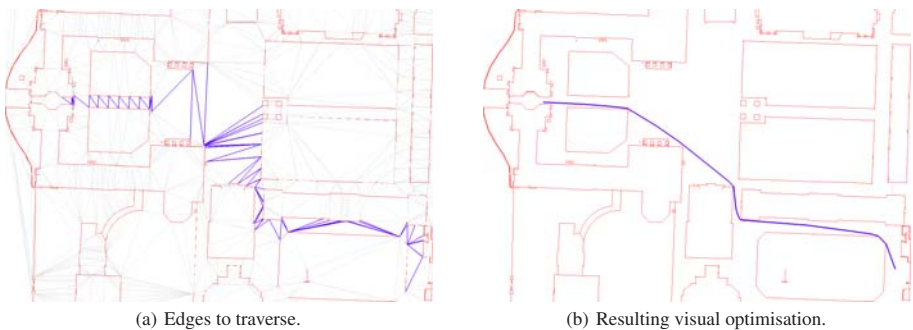
Fig. 2. Path planning in Trinity College Dublin. The underlying subdivision is represented with traversable gray edges and obstacle red edges; the resulting path is shown in blue.
