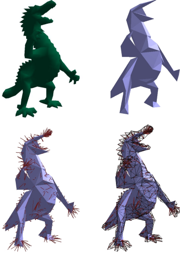
Figure 1: Top left figure shows a dense mesh whose deformations are steered by a coarser mesh, top right. Rigid links are used to link both meshes, bottom.
