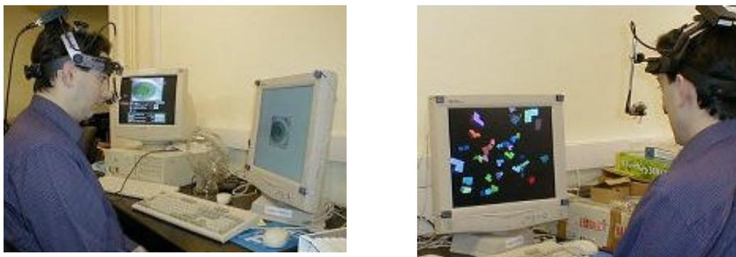
**Figure 4: An eye-tracker is used to determine the viewer's point of fixation**
