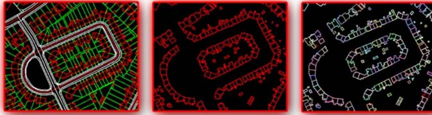
Figure 1: Extracting building footprints from GIS data (left). Layer containing buildings is first chosen by the user (middle), while buildings are then extracted by finding loops in the data (right).
