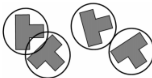
(a) intersection at time t_0 (b) after backtracking to "collision time"
